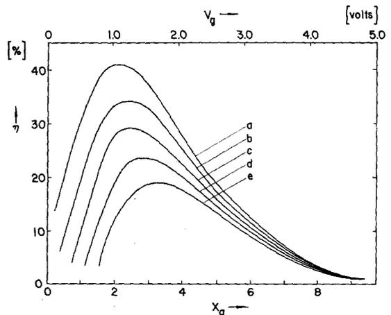
Fig. 5. Efficiency  $\eta$  for a blackbody solar cell at  $T_c=300^\circ\text{K}$ , with sun at  $T_s=6000^\circ\text{C}$ , as a function of energy gap for different values of the parameter  $f$ : curve (a)  $f=1$ ; (b)  $f=10^{-3}$ ; (c)  $f=10^{-6}$ ; (d)  $f=10^{-9}$ ; (e)  $f=10^{-12}$ .
