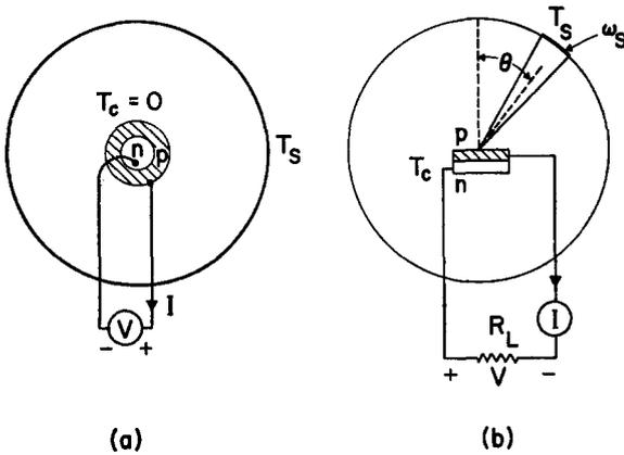
FIG. 2. Schematic representation of the solar battery considered. (a) A spherical solar battery surrounded by a blackbody of temperature  $T_s$ ; the solar battery is at temperature  $T_c=0$ . (b) A planar cell irradiated by a spherical sun subtending a solid angle  $\omega_s$  at angle of incidence  $\theta$ .
