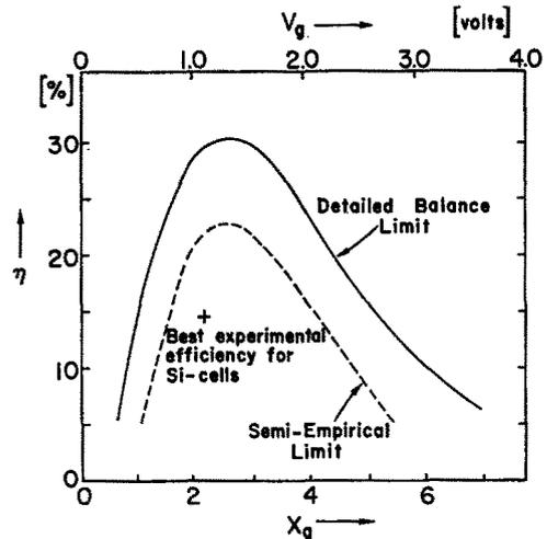
FIG. 1. Comparison of the "semieempirical limit" of efficiency of solar cells with the "detailed balance limit," derived in this paper. + represents the "best experiment efficiency to date" for silicon cells. (See footnote 6.)
