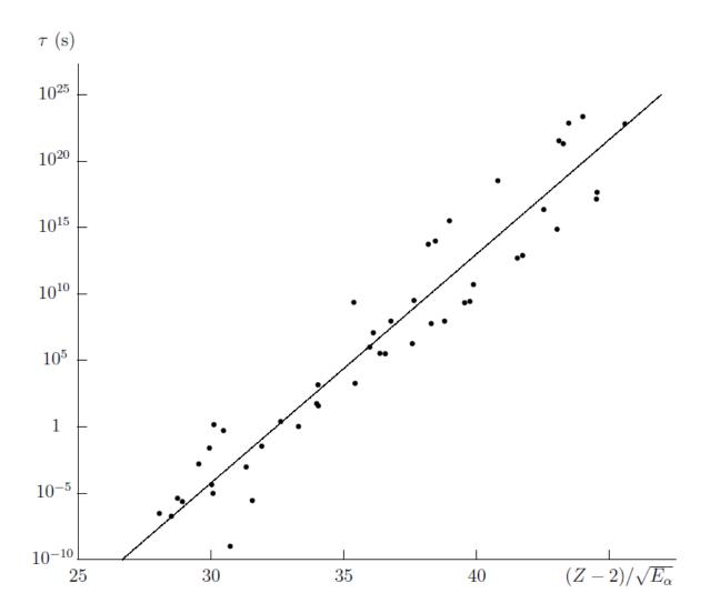
${\it E}_{\alpha}$  is the kinetic energy of the  $\alpha$  particle in MeV
