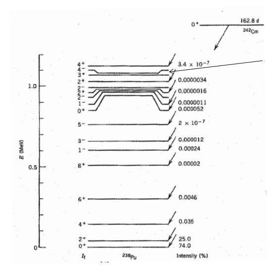
The 3<sup>+</sup> state is forbidden by the parity selection rule  $\rightarrow 0 \rightarrow 3$ decay must have  $\ell_{\alpha} = 3 \rightarrow$  the parity has to change
